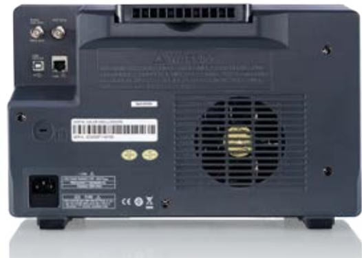
USB Host, USB Device (USBTMC), LAN(VXI-11), Pass/Fail and Trigger Out
