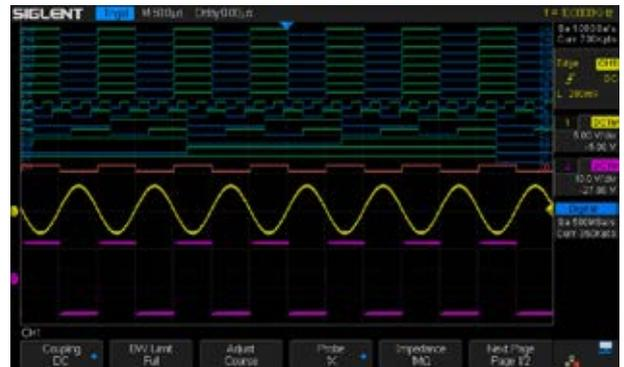
2 analog channels plus 16 digital channels enables users to acquire and trigger on the waveforms then analyze the pattern, simultaneously with one instrument.
