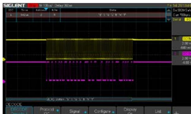
SDS1000X-E displays the decoding through the events list. Bus protocol information can be quickly and intuitively displayed in table form.
