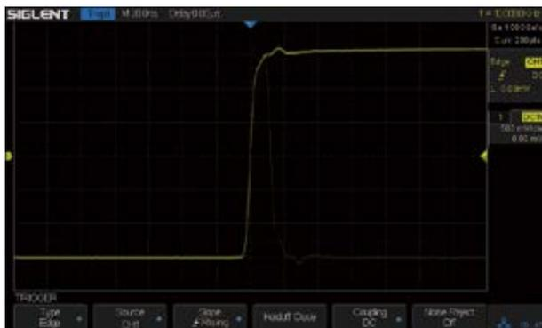
Up to 60,000 frames / second waveform capture rate, the oscilloscope can easily capture the transient events or low-probability events
